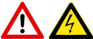
**HAZARDOUS VOLTAGE.** *Electrical power must not be connected until all wiring and limit switch adjustments have been completed. Once the power is supplied to the unit, precautions must be taken if the cover is not mounted on the actuator.*
