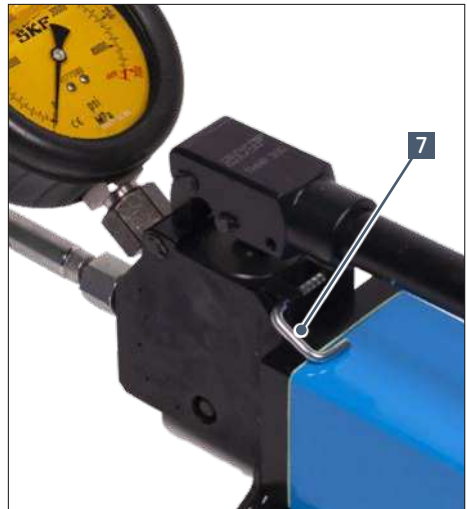
Fig.7 – Stop lever clip in released position
