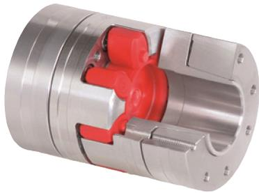
**ROTEX® GS** is a three-part, axial plug-in coupling backlash-free under prestress. It impresses even with critical applications by its backlash-free power transmission, its stiffness which is each adapted to the application and its optimum damping of vibrations. Using this principle provides for significant options of assembly optimizing the assembly times in production.
