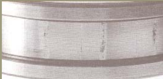
Inner ring of a cylindrical roller bearing damaged by vibrations. The damages occurred when the bearing was not rotating. It is clear, by seeing the littlest tracks between the more marked tilts (with corrosion on the bottom), that the ring has changed its position for small periods
