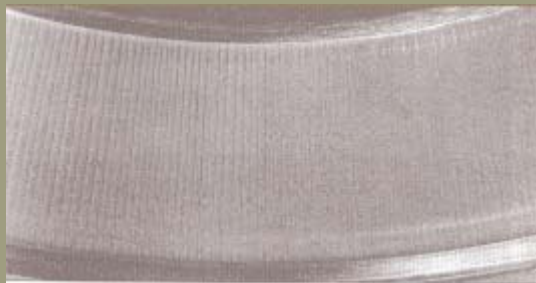
Outer ring of a tapered roller bearing damaged by the vibrations during functioning.
